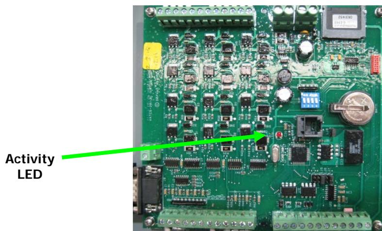
After locating the Control Board, all cables linking it to the rest of the sign should have their positions carefully noted and then be disconnected by undoing the terminal screws securing the cables to the board.
