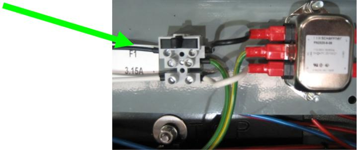
The remaining fuse is also a slow blow/Time Delay type rated at 10 Amps located on the DIN Rail as shown below:
