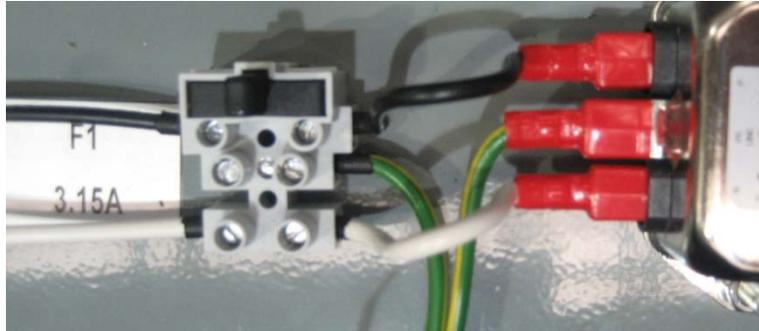
Strip back each core 6mm (1/4") and connect the earth core into the terminal marked  $\perp$  (the middle terminal). Connect the live core to the live fused terminal and the neutral core into the neutral terminal. Ensure the fuse in the black fuseholder is the correct rating (3.15A slow blow) and refit to the screw terminals.
