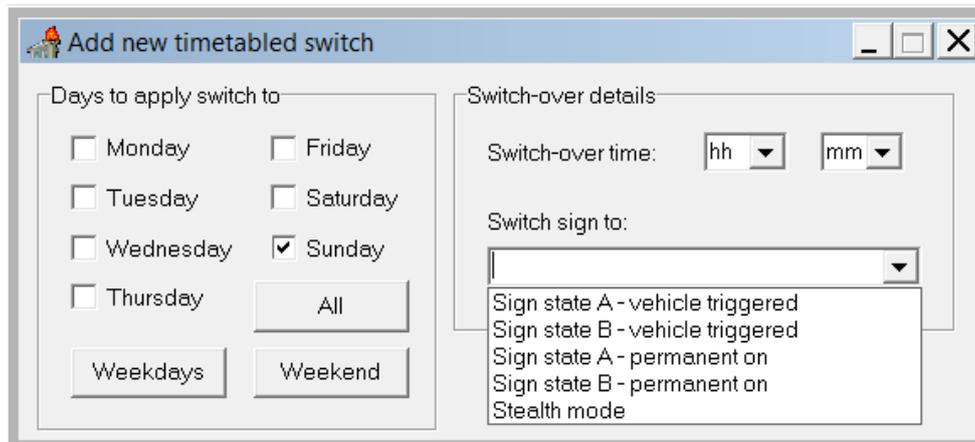
The settings required are Sign State A – Permanent On to set the time the sign illuminates and Stealth Mode to turn the sign off.
