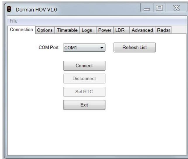
Once the connection is made the screen will show the legend 'Connected' and the Set RTC and Disconnect buttons will become active.
